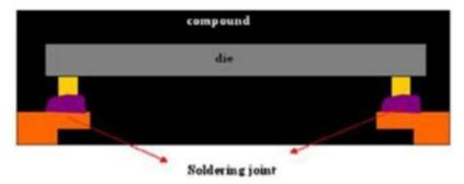
Flip-chip chip scale package (FC CSP) construction utilizes the flip chip bumping (with solder bump or Cu pillar bump) interconnection technology to replace the standard wirebond interconnect. It allows for a smaller form factor due to wire loop reduction and area array bumping. FC CSP includes the substrate or leadframe type solution making an attractive option for advanced CSP application when electrical performance is a critical factor.
