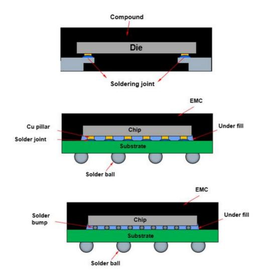
FC Chip Scale Package (FC CSP) construction utilizes the flip chip bumping (with solder bump or Cu pillar bump) interconnection technology to replace the standard wire-bond interconnect. It allows for a smaller form factor due to wire loop reduction and area array bumping. FC CSP includes the substrate or leadframe type solution making an attractive option for advanced CSP application when electrical performance is a critical factor.
