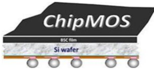
Wafer-level CSP (WLCSP) is the technology of packaging an integrated circuit at wafer level. WLCSP is essentially a true chip scale package (CSP) technology, since the resulting package is practically of the same size as the die. WLCSP has the ability to enable true integration of wafer fab, packaging, test, and burn-in at wafer level in order to streamline the manufacturing process undergone by a device start from silicon wafer to customer shipment.
