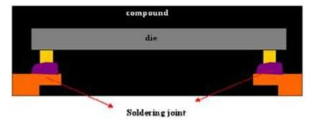
Flip-chip chip scale package (FC CSP) construction utilizes the flip chip bumping (with solder bump or Cu pillar bump) interconnection technology to replace the standard wirebond interconnect. It allows for a smaller form factor due to wire loop reduction and area array bumping. FC CSP includes the substrate or leadframe type solution making an attractive option for advanced CSP application when electrical performance is a critical factor.
