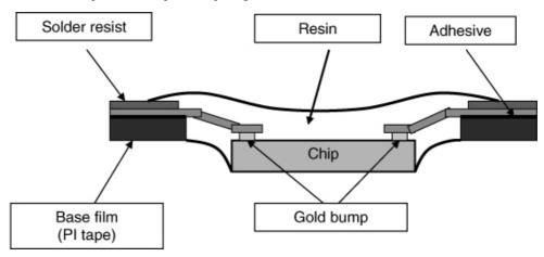
The tape carrier package assembly process involves the following steps:
