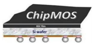
Wafer-level CSP (WLCSP) is the technology of packaging an integrated circuit at wafer level. WLCSP is essentially a true chip scale package (CSP) technology, since the resulting package is practically of the same size as the die. WLCSP has the ability to enable true integration of wafer fab, packaging, test, and burn-in at wafer level in order to streamline the manufacturing process undergone by a device start from silicon wafer to customer shipment.
