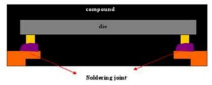
Flip-chip scale package (FC CSP) construction utilizes the flip chip bumping (with solder bump or Cu pillar bump) interconnection technology to replace the standard wirebond interconnect. It allows for a smaller form factor due to wire loop reduction and area array bumping. FC CSP includes the substrate or leadframe type solution making an attractive option for advanced CSP application when electrical performance is a critical factor.
