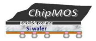
Wafer-level CSP (WL CSP) is the technology of packaging an integrated circuit at wafer level. WL CSP is essentially a true chip scale package (CSP) technology, since the resulting package is practically of the same size as the die. WL CSP has the ability to enable true integration of wafer fab, packaging, test, and burn-in at wafer level in order to streamline the manufacturing process undergone by a device start from silicon wafer to customer shipment.
