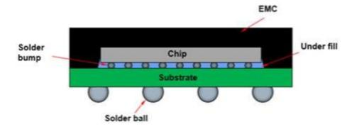
Flip-chip chip scale package (FC CSP) construction utilizes the flip chip bumping (with solder bump or Cu pillar bump) interconnection technology to replace the standard wire-bond interconnect. It allows for a smaller form factor due to wire loop reduction and area array bumping. FC CSP includes the substrate or leadframe type solution making an attractive option for advanced CSP application when electrical performance is a critical factor.
