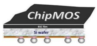
Wafer-level CSP (WLCSP) is the technology of packaging an integrated circuit at wafer level. WLCSP is essentially a true chip scale package (CSP) technology, since the resulting package is practically of the same size as the die. WLCSP has the ability to enable true integration of wafer fab, packaging, test, andburn-in at wafer level in order to streamline the manufacturing process undergone by a device start from silicon wafer to customer shipment.
