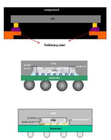
Flip-chip chip scale package (FC CSP) construction utilizes the flip chip bumping (with solder bump or Cu pillar bump) interconnection technology to replace the standard wire-bond interconnect. It allows for a smaller form factor due to wire loop reduction and area array bumping. FC CSP includes the substrate or leadframe type solution making an attractive option for advanced CSP application when electrical performance is a critical factor.
